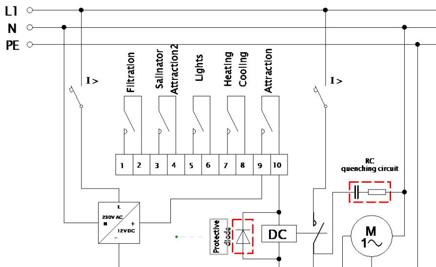
This is the recommended output connection of the Vario DIN Module for connection of inductive load inside a breaker box (diagram is valid for one output = in this case the "Attraction" contact). Connect the other outputs with inductive load accordingly.
