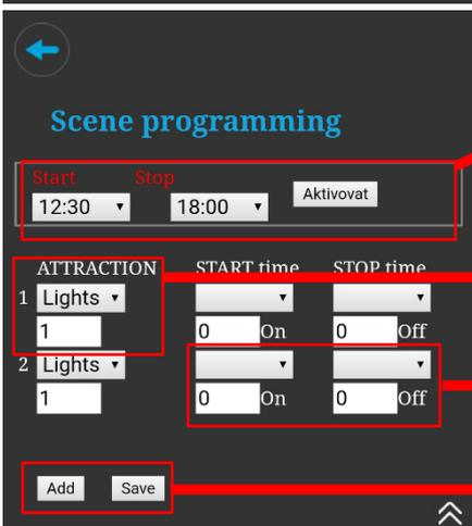
**Master scene time-frame** – the sequences may run only during this interval. Press **Activate** to initiate.
