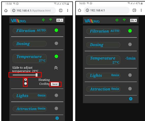
Relay output R4 of the DIN module could be configured for “Heating” (this case) or “Cooling”.
