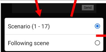
Select the function for setting – pre-programmed scenarios or next color (pulse). When Scenario is selected, enter the desired scenario position and press **Send**
