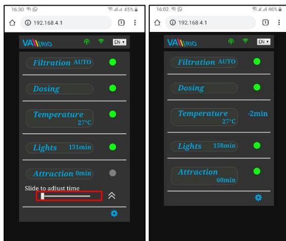
Relay output R5 of the DIN module is used for pool attraction with timer (+5 min. step). Operation timer can be set within the 0-120 minutes range. The same settings could be applied also for the R2 relay in Attraction2 mode.
