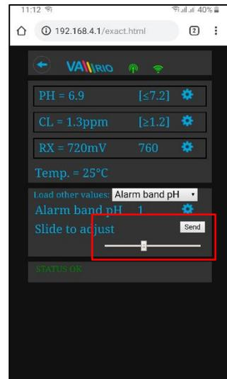
The alarm band settings shown above are for the pH. You can set the alarm bands also for the Redox (RX) and Chlorine (CL) parameters the same way. The default password for dosing adjustments is „1234“.
