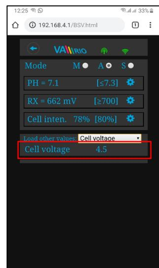
The adjustments and settings above are available for the pH parameter. Adjust the CL, RX values or alarm bands the same way. The salinity value can be displayed only if a salinity sensor is attached. Default password for all settings is "1234".
