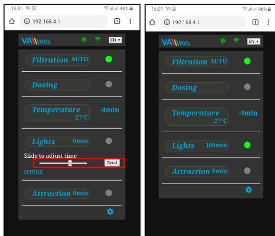
Relay output R3 of the DIN module is used for pool lights with timer (+5 min. step). Operation timer can be set within the 0-120 minutes range.
