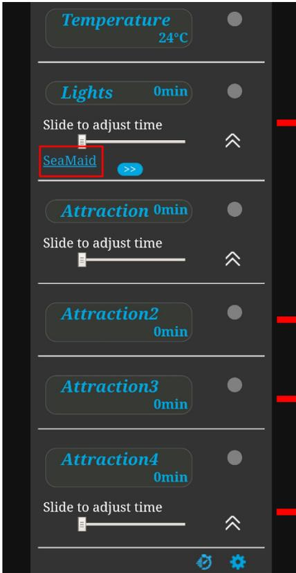
The Lights control panel allow she user to control either lights without DMX communication (SeaMaid, RGB Flat) or lights with DMX communication (Adagio Pro, Hugo Lahme, Wibre). Enter the control menu by pressing the DMX (SeaMaid/RGB Flat button). Control functions are below.
