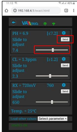
Adjust the Chlorine or Redox values the same way and confirm with Send
