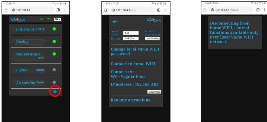
**TIP:** If the 192.168.4.1 page doesn't open, disable mobile data on your device. With concurrently enabled mobile data your device tries to connect over the Internet, not over local VARIO WIFI network.
