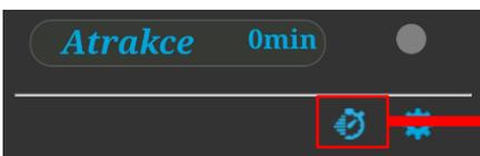
Press the „Stopwatch“ to enter the **sequence programming menu**. Here you can program sequences of various attractions combined with lights – even with lights of different colors.
